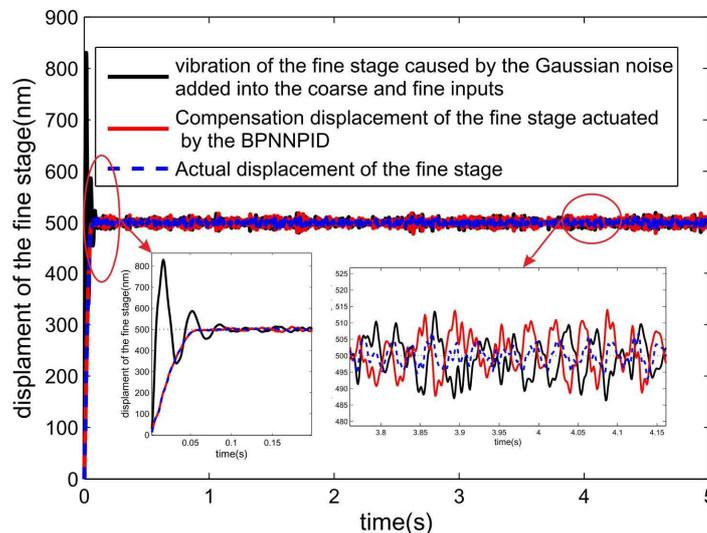
Figure 3. Simulation results of the BPNNPID for vibration suppression
