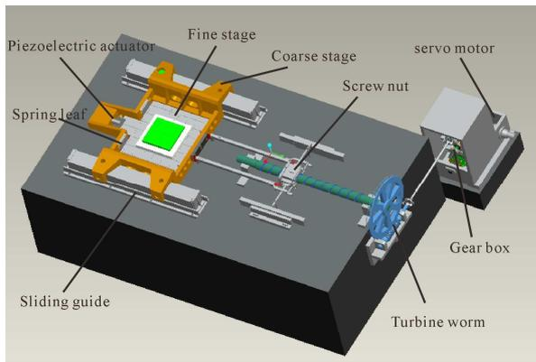
(a) Architecture of the positioning system
