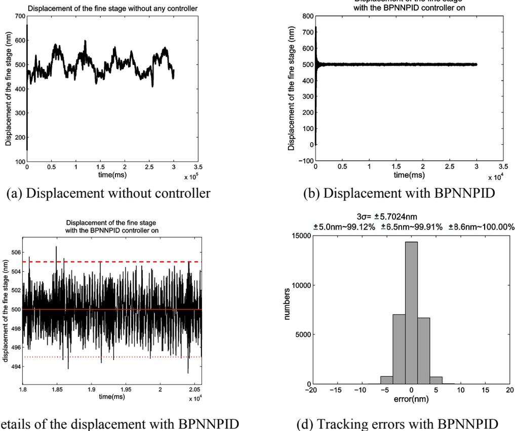
Figure 4. Results of the experiment with a reference step signal valued 500nm
