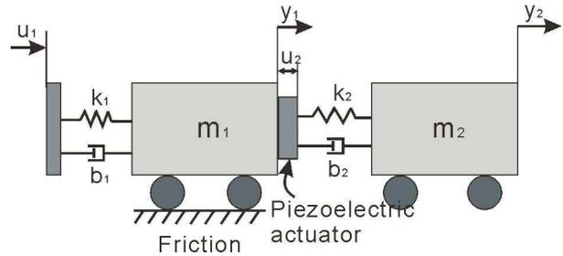
(b) Physical model of the positioning system
